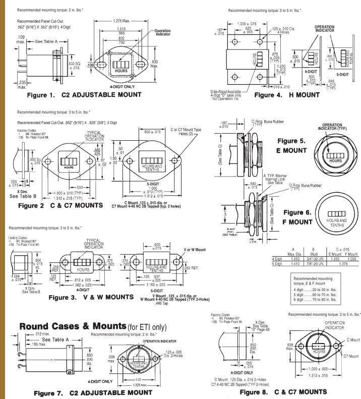
\*When mounting flanged units, it is recommended to distribute the mounting torque evenly across the mounting surface. Each mounting screw should be alternately tightened about one quarter to one half turn until the recommended torque is attained on each screw. The mounting surface should be flat to avoid exerting stress on the body of the unit.
